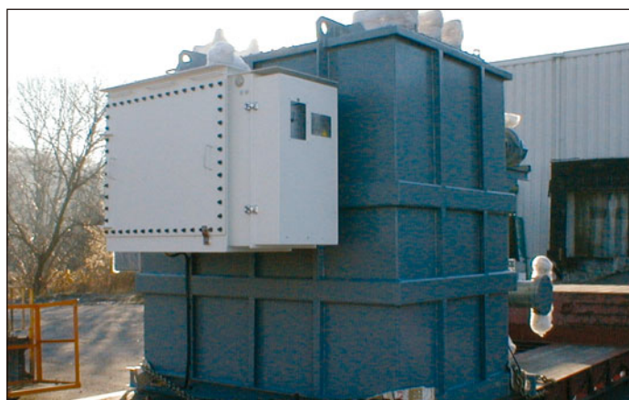
3200 KVA Furnace Transformer with OLTC
