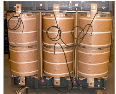
2100 KVA 12 Pulse Core & Oil
