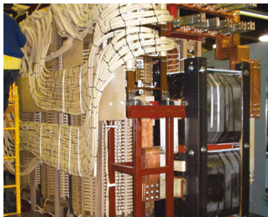
16 MVA Rectifier Core & Coil
