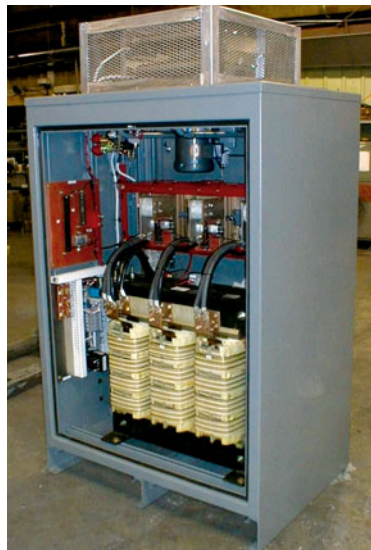
Crane Duty Supply with Regen
