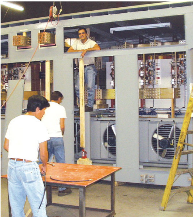
30 KA @ 233 VDC 12 pulse supply - Bleach Supply
